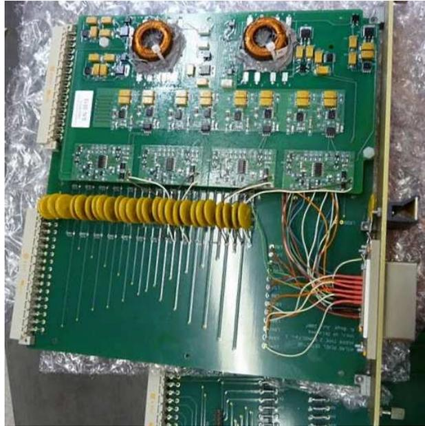
Figure 2: A sample Current Measurement Board.
