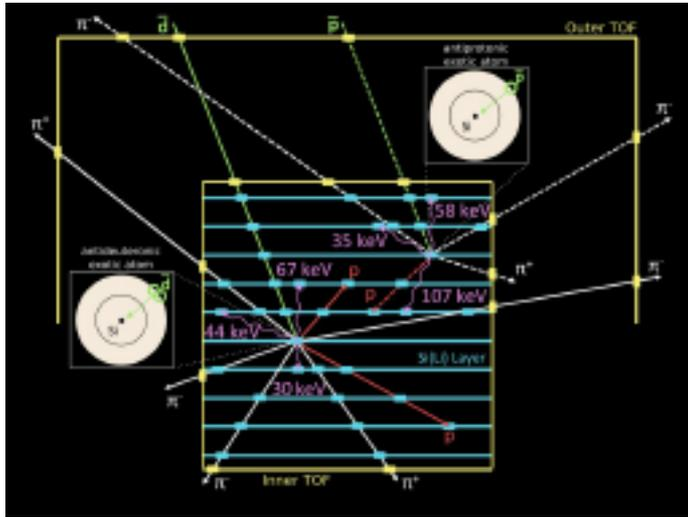
Detection of cosmic anti-nuclei using TOF as antiparticle target, de-excitation x-ray spectrometer, and antinucleus  $dE/dx$  tracker
