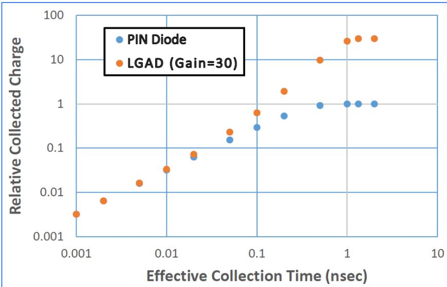
Study of fundamental properties of impact ionization and solid-state charge collection suggests that LGADs are advantageous to frame rates up to 10+ GHz
