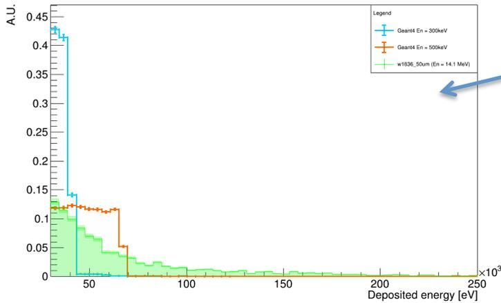
LGADs can be used to detect neutrons from 300 keV up to few MeV in high flux conditions with 20-30 ps resolution. Simulations predict possible sensitivity also for energy range [15-140] keV
