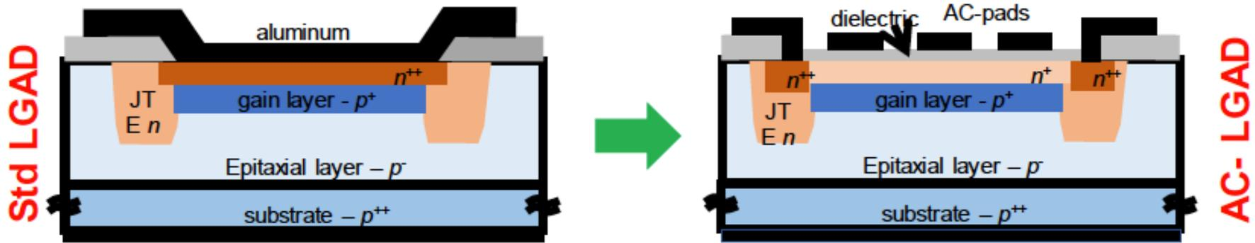
LGADs have been fabricated at BNL, and these formed the basis for AC-LGADs after modification of a few masks and tuning of the process flow.
