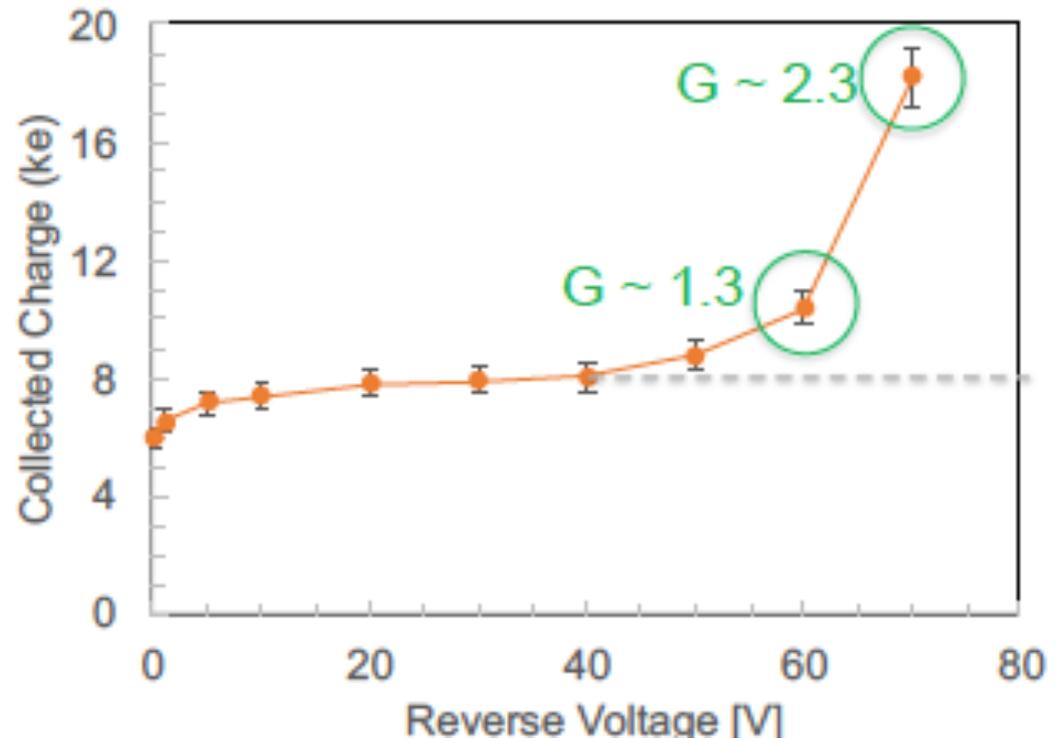
Gain up to  $\sim 2$  observed in 1N-1P devices with  $I_{\text{leakage}}$  and capacitance comparable to traditional pitch devices; study ongoing to understand spatial distribution of the multiplication.
