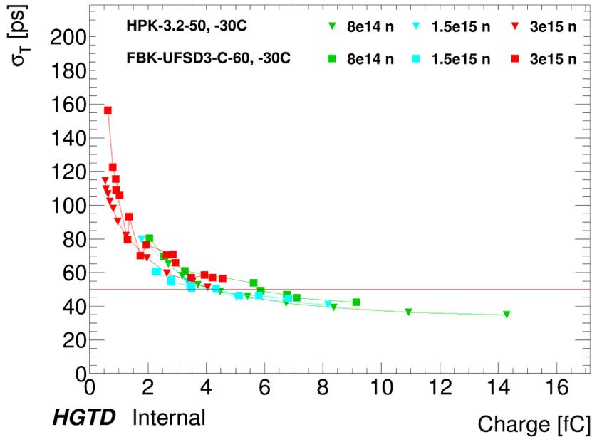
Time resolution vs. collected charge is mostly independent of radiation damage up to  $3 \times 10^{15}$  neq with gain (8-10) and time resolution (50-60 ps).
