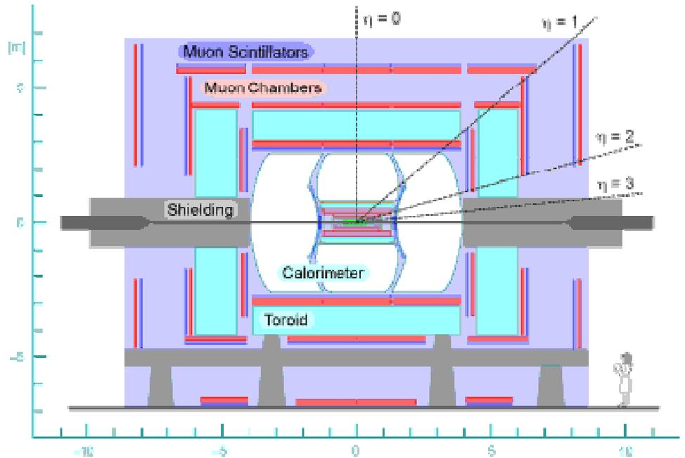
■ *calorimeters* LAr + U, Cu, or stainless cover  $6 \lambda_A$  with  $\Delta\eta \times \Delta\phi = 0.1 \times 0.1$  over  $|\eta| < 1.1$  and  $1.5 < |\eta| < 4.2$ .
