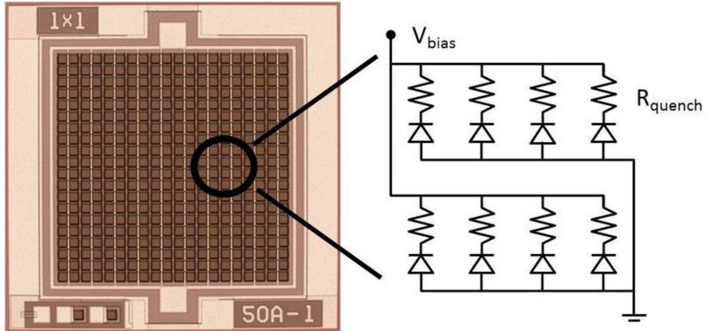
Single photon sensitive structures built from an array of sequentially connected avalanche photodiodes. Each APD is coupled through a quenching resistor and operates in Geiger mode, providing a dynamic range from 1 to 1000 photons per  $\text{mm}^2$ . Can be used in a compact calorimeter in a high magnetic field.
