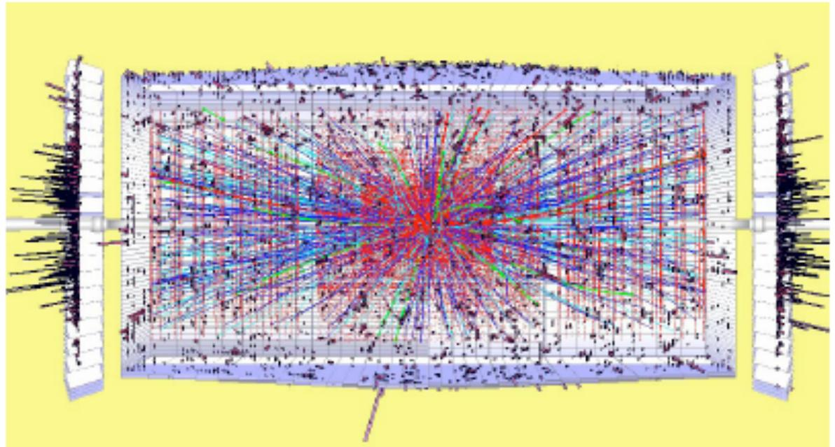
SLHC,  $L = 10^{35} \text{ cm}^{-2}\text{s}^{-1}$ ,  $\sim 200 \text{ MBE}$
